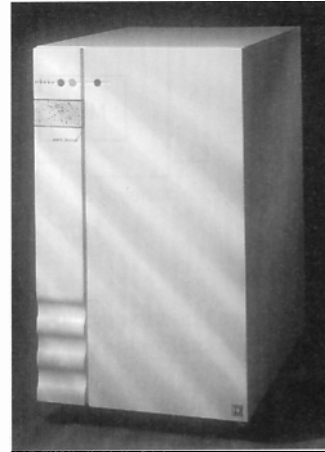
Figure 29.17b This 18 kVA, 120/208 V, 3-phase, 60 Hz on-line UPS generates an output of 120/208 V, 60 Hz at output power factors ranging from 0.7 lagging to 0.7 leading. The THD is less than 5 percent, even with nonlinear loads. The full-load efficiency is about 90 percent. The low noise level and small size are due to the high switching frequency ( \approx 16 kHz) of the IGBT inverter. If power is interrupted, or exceeds the input tolerance window, the internal battery supplies power to the inverter for up to 10 minutes with no interruption to load. (Courtesy Square D/Gruppe Schneider)
